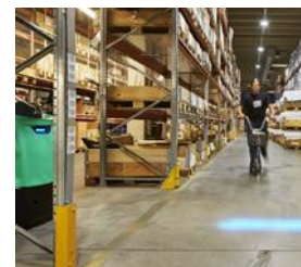
Blue point safety light towards driving direction.
