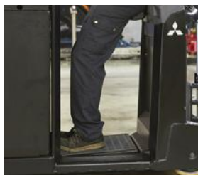
Suspended operator's platform.
