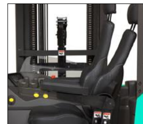
Suspension seat with tilting backrest
