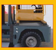
Strong, reliable and refined, the GX provides excellent productivity and safety for long load users. On the deck, there are two durable options - a toughened hardwearing composite cover, or checkerplate steel decks with hard-wood timber bearers.
