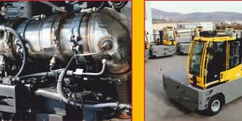
The GX Series features two powerful engines - the TCD 55kw Deutz Stage V diesel engine with DPF & DOC, without Ad the panoramic glass panel on the new cabin. accurate mast travel. A bespoke valve Blue, or the powerful 85kw option with DPF, DOC, and Ad Blue. The reliable hydrostatic transmission, load sensing, joystick control, and full road-legal LED lighting make this the market leader in engine sideloaders.
