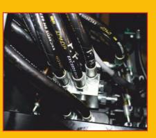
worked with our valve bank supplier to improve its performance, allowing movements characteristic only to sideloaders and new options, such as the choice of electronic or manual joysticks. Two Bosch & Rexroth hydrostatic wheel motors are used in conjunction with piston pumps with variable displacement.
