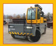
The guiding principle is a robust and simple construction combined with compact dimensions for maximum possible manoeuvrability and service-friendliness. With their 16.00-25 tyres, these sideloaders remain the most compact - and thus most manoeuvrable - in their load class.
