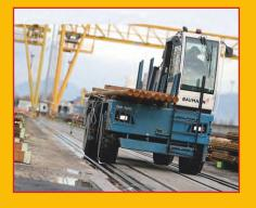
All the advantages of the Baumann sideloaders, such as the automatic stabilization system or the hydraulic bushings under the cab, can be found in this series as standard.
