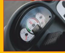
Our clear, simple dashboard puts all essential information at your fingertips. The centre console indicates warnings and diagnostics information on key entry and startup. Pre-operation checklists can be incorporated via the Optafleet system and as standard the seat switch will also prevent operation without an operator
