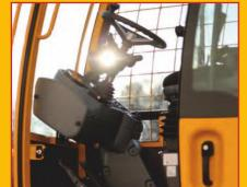
Changes in materials and advances in toughened glass allowed us to reconfigure the glass panel on the new cabin. The result is a more sturdy design, together with more sensitive control via a joystick or mini-levers option.
