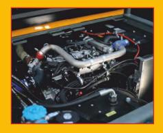
This low-emission optimized powerful diesel 55kw HATZ diesel engine is Stage V compliant with DPF and DOC and no Ad Blue. A Bosch Rexroth hydrostatic transmission, Poclain hydrostatic wheel motors and piston pump with variable displacement complete the high specification drive train.
