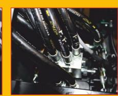
The HX utilises a bespoke steering axle and flow matching hydraulic system. Through closed-loop control, the hydraulic pressure is adjusted depending on the load, saving energy and improving efficiency. Hydraulic joysticks come as standard with optional hydraulic levers available.
