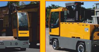
Over 8 hours continuous run time, panoramic cabin, load sensing, joystick control, full road-legal LED lighting and precise mast control makes this durable machine one of the most productive and energy-efficient ever made.
