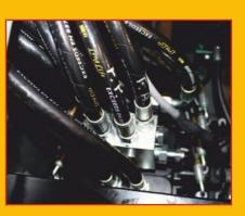
The ELX utilises a bespoke steering axle and flow matching hydraulic system. Through closed-loop control, the hydraulic pressure is adjusted depending on the load, saving energy and improving efficiency.
