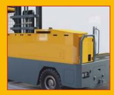
Electrics offer zero emissions, are cheaper to run and maintain, as well as offering a better operator environment. Noise and cost savings will also benefit long-established companies that are under pressure to cut emissions and noise pollution by neighbours and legislators. Lithium-ion battery options are also available.
