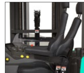
Suspension seat with tilting backrest
