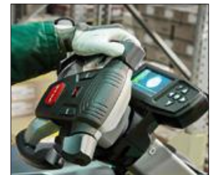
Multifunctional steering wheel with optional color display.
