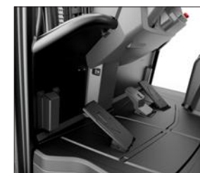
Dual pedal system - forward and reverse. (Option)
