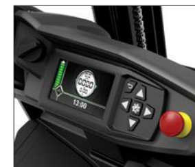
Multifunctional colour display (hourmeter, BDI etc.)
