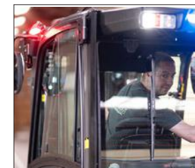
Blue point and red line safety lights
