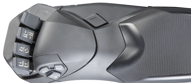
ErgoCentric adjustable armrest with integrated fingertip control
